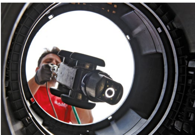
Diameter of the AQUABOX CUBE extension tube: 400 mm Maximum shaft depth: 6,5 m Tunnel section, width x height: 17 x 30 cm
