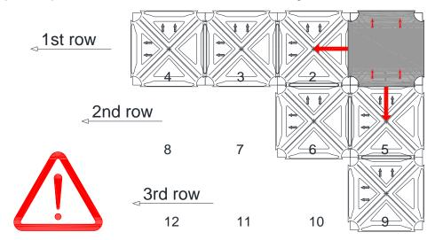
Before beginning the installation of the elements, it is recommended that you consult Geoplast's design tables in order to position the elements properly. For proper installation, in compliance with safety regulations, please refer to the installation manual.
