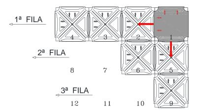
Before beginning the installation of the elements, it is recommended that you consult Geoplast's design tables in order to position the elements properly. For proper installation, in compliance with safety regulations, please refer to the installation manual.
