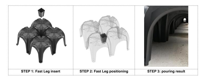
Thanks to the "Fast Leg" accessory, it will be possible - always for the heights 50, 55, 60, 65 and 70 cm - pouring the concrete in one-step. In this way, the casting operations become much simpler and faster and the site workers work in optimal conditions, without any possibility of laying error. The use of "Fast Leg" eliminates the need to insert the sealing ring.
