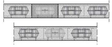
Figure 53 - shear reinforcement: longitudinal and transverse section
