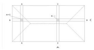
Figura 9 - representation of the strip method according to Hillerborg.
