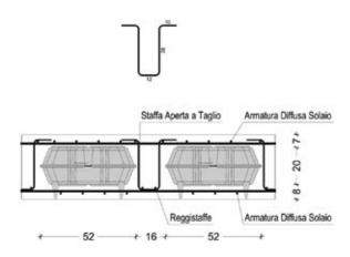
Figura 29 - shear- resistant open ties
