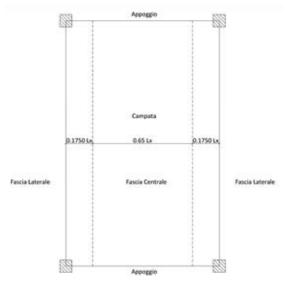
Figura 14 - diagram for the calculation of design moments in the y direction - width of the central and lateral strips.
