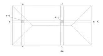
Figura 22 - representation of the strip method according to Hillerborg
