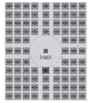
Figura 7 - non-lightened concrete area dimensions - capital
