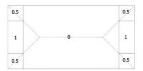
Figura 11 - possible distribution (B) in a rectangular plate leaning on the boundary.
