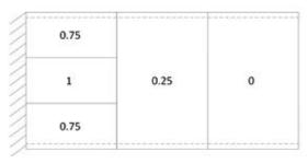
Figura 25 - possible redistribution in a rectangular plate with constraints to mixed
