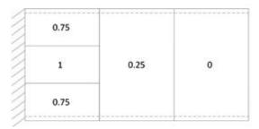
Figura 12 - possible redistribution in a rectangular plate with constraints to mixed boundaries.
