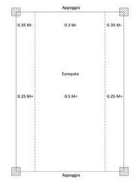
Figura 15 - diagram for the calculation of the design moments - moments of competence of each strip.
