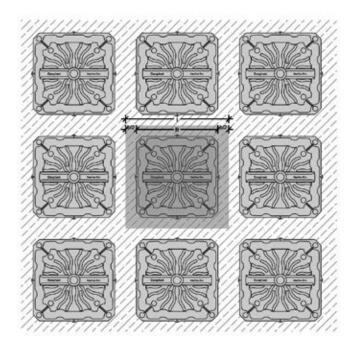
Figure 76 - overall surfaces of thermal resistances in parallel
