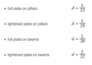
The minimum size of the upper and lower slabs is constrained by minimum covering requirements to be secured to the bars. Inside the slab the minimum reinforcement covering required by the regulations must be ensured for the category of exposure relating to the calculation hypotheses made, plus the two diameters of the basic reinforcement in the two directions.
