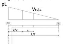
$$\frac{L_{x/y}}{2} : p \cdot L_{x/y} = \left(\frac{L_{x/y}}{2} - \frac{c_{x/y}}{2} - x\right) : V_{Rd}$$
