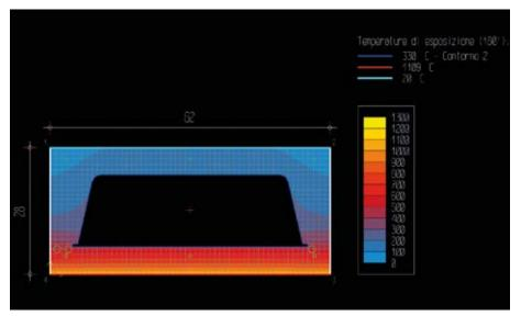
Figure 68 - calculation of thermal conduction over time for application of standardized temperature T (° C, t) curve
