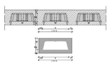
Figura 18 - section type - calculation of the reduction coefficients
