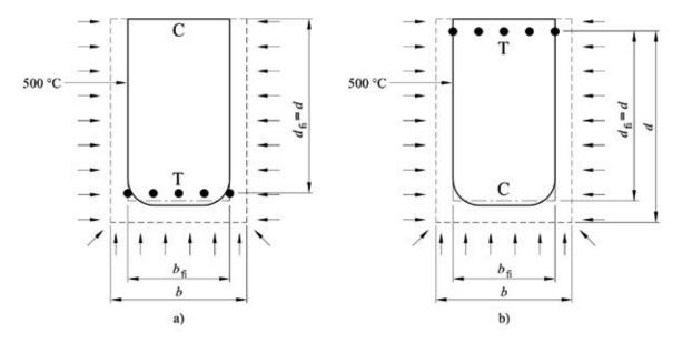
Figure 72 - reduction of the section subject to fire
