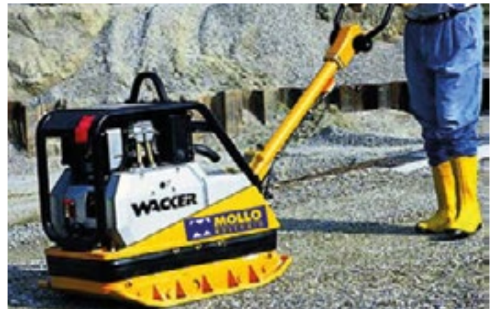
Figure 19 - Compacting phase of the covering material
