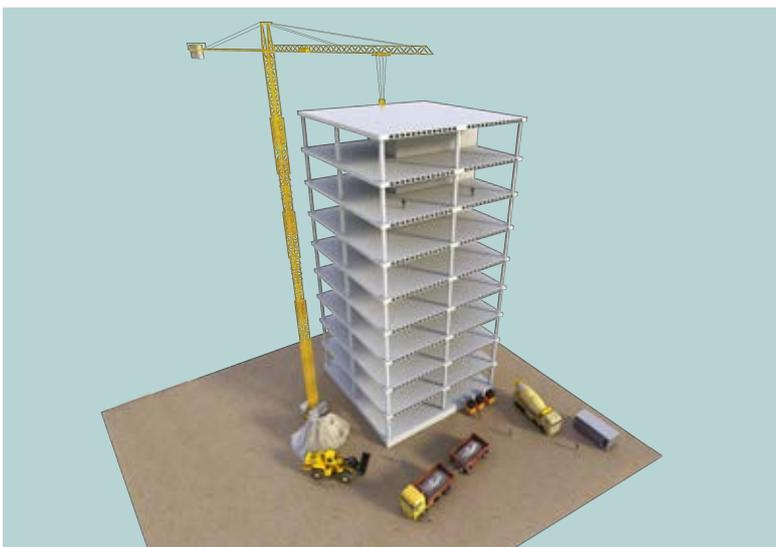
Geoplast void-former solutions reduce the weight of roof slabs, improving the seismic response of buildings and reducing the consumption of concrete and steel.
